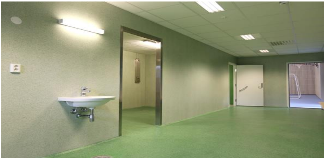
Acrylicon Wall System installed 2016 in a school in Norway, Melhus, Sør-Trøndelag. The floor installed with Acrylicon Flake System
